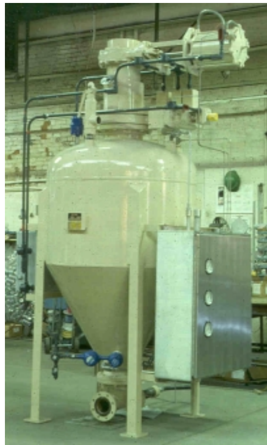
Transporter vessel for batch transferring of materials in true dense phase and low velocity conveying regimes
