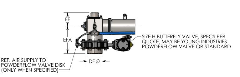
DISCHARGE SHOWN WITH OPTIONAL FLANGED CONNECTION AND BUTTERFLY VALVE.
