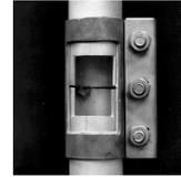
**Pinch clamps** - Available in several types, typically containing a gasket that wraps around the pipe joint. A shell is then clamped around the gasket with bolts or toggle
