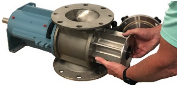
Rotor Slides Off Shaft C.
