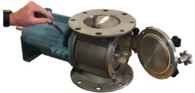
Pin Removed From Rotor Shaft To Allow Rotor And Shaft Seal Removal B.
