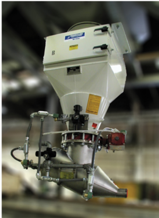
Model PI310-125 Multi-phase product Pump for conveying powder from Bulk Bag Unloading Station
