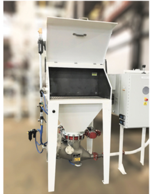
Model FBD10-3-C Filter Bag Dump Station with PI 308-125 Multi-Phase Product Pump
