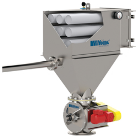
Low headroom HW Filter Receiver uses horizontal filter bags. A Model HC Rotary Valve is used as an airlock to discharge powder to the process below
