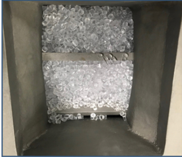
Clipping that Occurs in Standard Drop Through Rotary Valve
