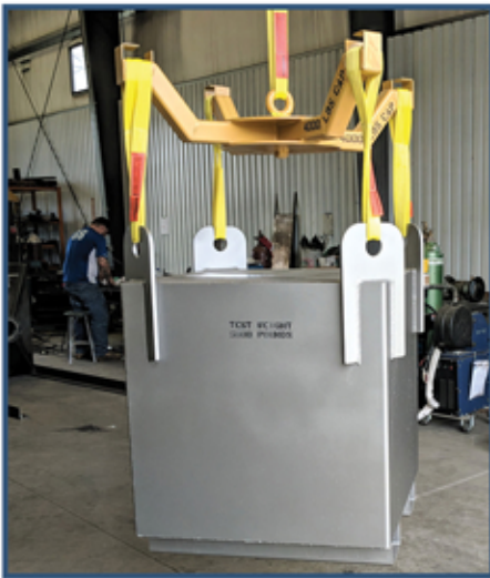
Load Testing Low Profile Lifting Bracket
