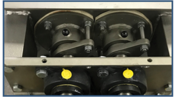
Packing gland seals with air purge connections and outboard bearings
