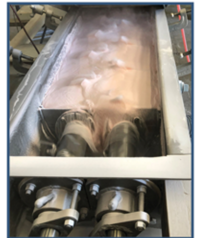
Weir Plate in position while mixing powders
