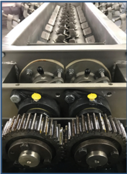
AGMA Spur Gears at discharge end of mixer
