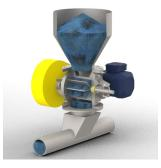
Metering: Valve is volumetrically controlling the flow of product.
