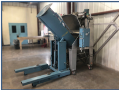
Dumper Chute Tipped Into Bag Dump Station
