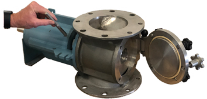
B. Pin Removed From Rotor Shaft To Allow Rotor And Shaft Seal Removal
