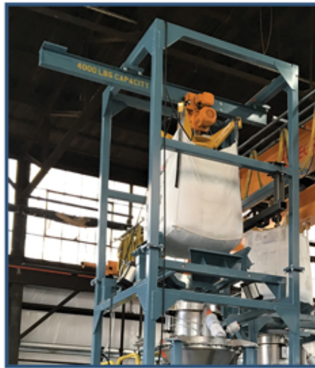
Unloading Frame With Low Profile Lifting Bracket
