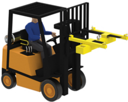
Lifting Bracket Placed on Fork Lift
