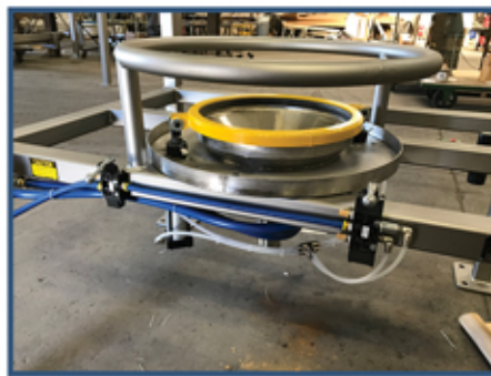
Clamp Ring Assembly With Support Ring
