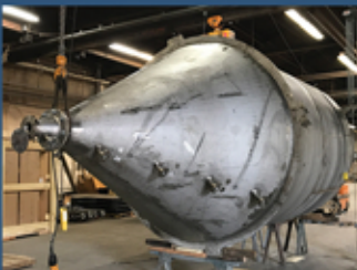
400 cu. ft. Holding Hopper with TransFlow® Lining (See Young Bulletin 265-200-1) Constructed of 304L S/S Operating pressure – 135 psig Build per ASME Code Section VIII, Div 1 ASME "U" Stamped
