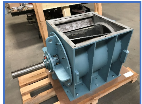
Completed valve fully assembled
