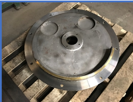
End plate after modifications
