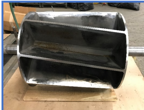
Modified rotor with stellite on tips and shrouds
