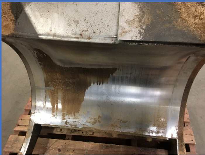
Hard chrome plated bore worn and grooved
