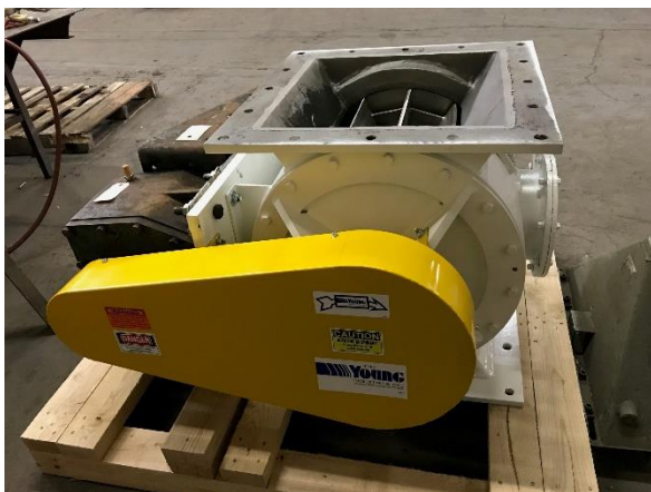
Inlet view of valve with new rotor installed
