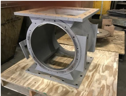
Rotary Valve housing after bead blasting
