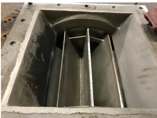
Inlet view of valve with new rotor installed
